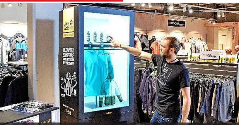
"The HYPEBOX 43" InWall is a ready-to-go Transparent Display solution designed for retail spaces and event locations. The whole construction is made to be integrated into walls - while the smart opening system makes it possible to service the unit & change products from the front."
